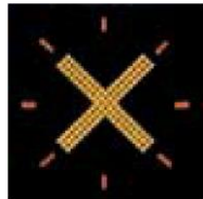
The FLASHING AMBER Cross is a caution signal to indicate possible obstruction ahead although the lane is open to vehicles. Drivers must slow down and be prepared to change lane
