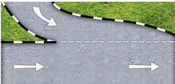
(h) Broken White Line at Accelerating Lane
