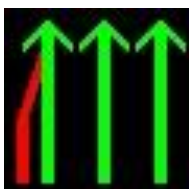
Lane Reduction (Obstruction at lane 4. Slow down. Drive carefully. Get ready to change lane if necessary)
