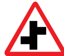
Staggered junction (Slow down. Beware of vehicles from the right and left)
