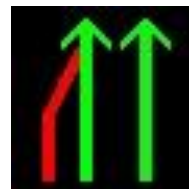
Lane Reduction (Obstruction at lane 3. Slow down. Drive carefully. Get ready to change lane if necessary)
