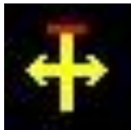
Right & Left Turns Only (Arterial Road – Through lanes closed ahead)
