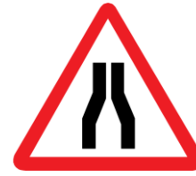
Road narrows on both sides (Slow down. Do not overtake, make a U-turn or park your vehicle)
